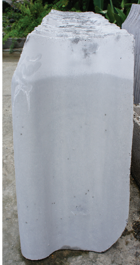
Left photo: MCR tiles stacked upright for air curing. Top right photo: The workers trained to make MCR tiles came from Manicani Island. Bottom right photo: The warehouse in Brgy. Canawayon where construction materials for the Homonhon housing project will be stored is still being constructed.
