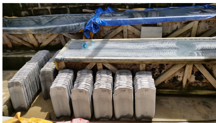
Production of MCR tiles are made in the Guiuan office of TAO-Pilipinas
