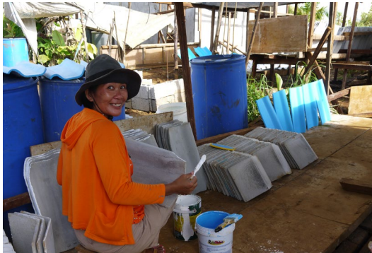
Shelter beneficiaries paint their own micro concrete roof tiles that will be used in their houses.
