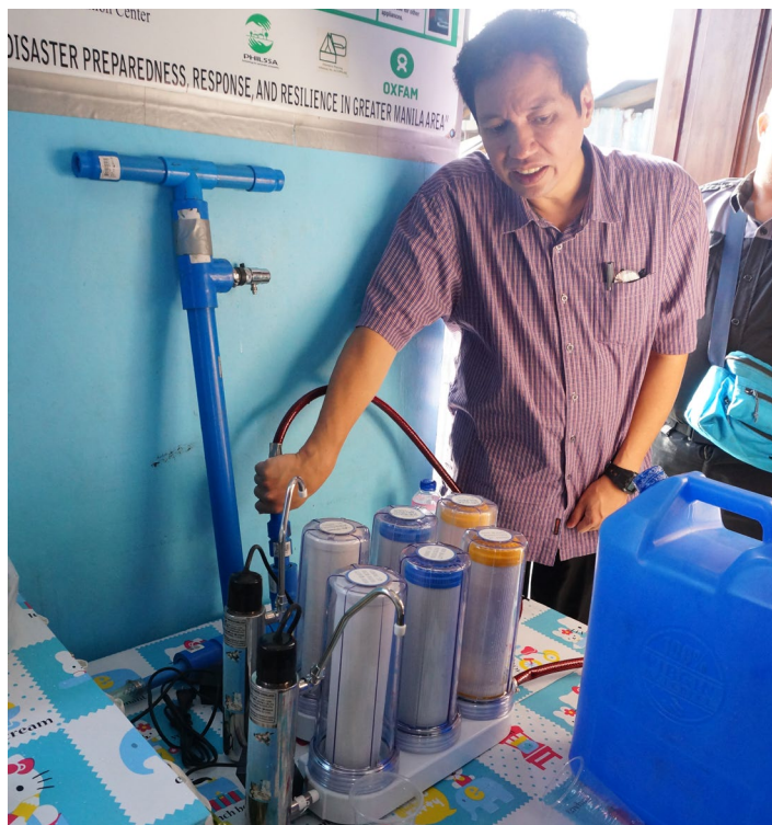
Mr. Carlos Oppus, director of AIC, checks the solar powered filtration system of the rainwater harvesting system that AIC helped set-up together with DRCHOA.
